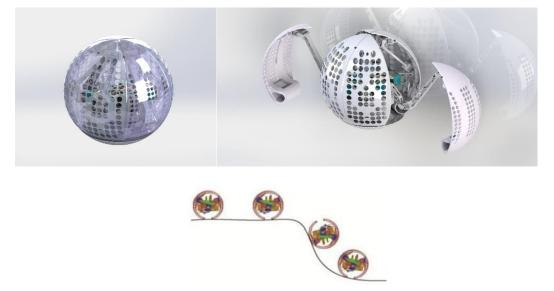
In the robot's crawling mode, the robot switches to hexapod mode to climb over the obstacle using leg movements. This mode is mainly used for climbing and rough road travel.
